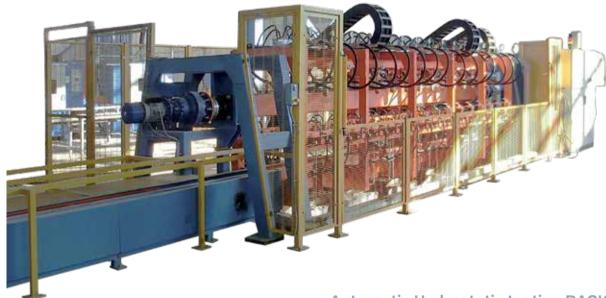
**Automatic Hydrostatic testing RACK**
