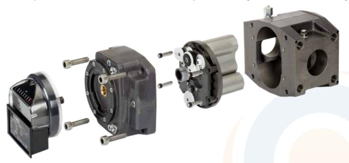
The use of a cartridge (pre-calibrated) and the accessibility of the front and rear bearings without the need for removing the timing gears, make the FMG series of rotary meter unique in terms of repair. Any repair shop can repair or re-condition the meters without special skills and tools. When regulation permits, a new, calibrated cartridge can be installed.
