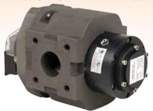
always accurate unless the rotors become jammed. In reality, the rotary meter is a digital device, it runs and is accurate or it stops. The only drawback of a rotary meter is that when it stops (locks up), the gas flow is interrupted. As such, there is no security of supply unless precautions are taken.
