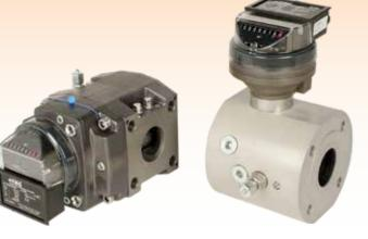
Installation of FMG rotary meters can be horizontal or vertical. Since the meter is designed for multi position, consideration need only be given to the arrows showing the flow direction. After the meter is installed, the index can be rotated to the correct position. The index can be rotated over 350°. FMG rotary meters can be metrological sealed to suit various conditions from total flexibility to highly tamper proof.
